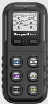
Flex 5 Diffusion Gas Detector Configured to Detect 6 Gases
