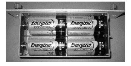
Replace the battery box and tighten thumbscrews.
