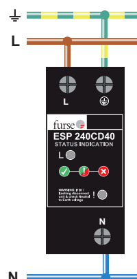
Parallel connection of ESP 240CD40 to single phase supplies (fuses not shown for clarity)
