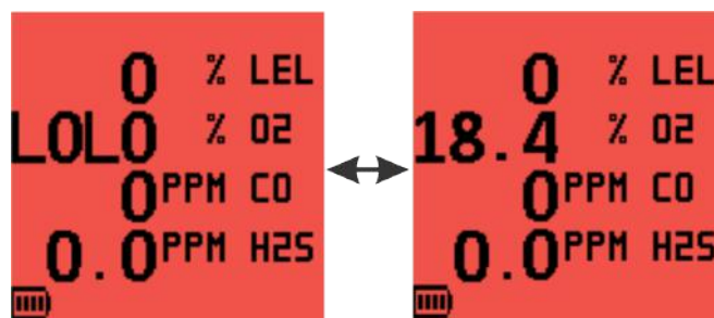
Figure 25: O 2 LOLO Alarm
