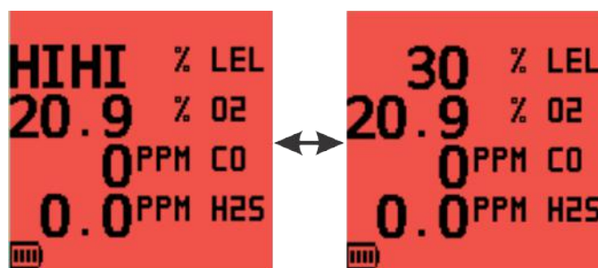
Figure 26: LEL HIHI Alarm
