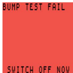
Figure 48: Bump Test Fail - Switch Monitor OFF
