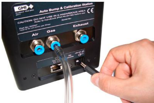
Fig. 2-8 Connect Power Supply to Station
