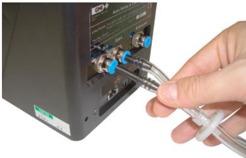
Fig. 2-7 Connect Air Tubing Adaptor to Station
