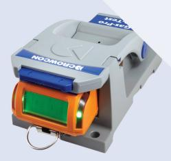
When used with a trigger regulator the cost of gas testing is low, taking only 12 seconds to complete a 5 gas test (CO,  $H_2S$ ,  $O_2$ ,  $CH_4$ ,  $CO_2$ )
