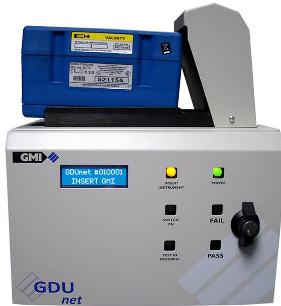
**Figure 1-1: Gas Delivery Unit (GDUnet)**
