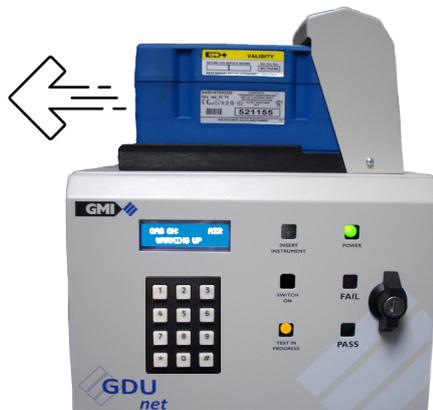
**Figure 3-27: Remove the instrument**
