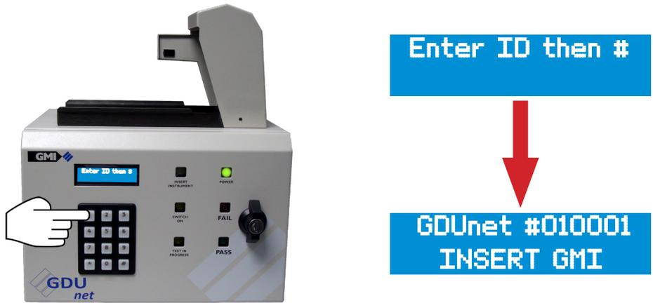
**Figure 3-23: Input the Operator ID**
