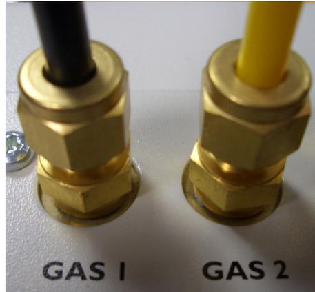
**Figure 2-8: Gases connected to GDUnet**
