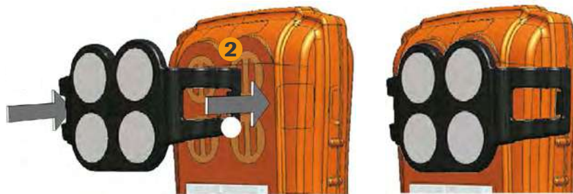
Figure 6: Fitting the external filter plate
