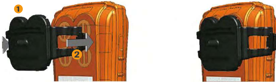
Figure 5: Fitting the calibration/bump test plate
