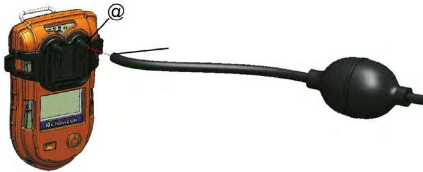
Figure 10: Attaching the Hand Aspirator
