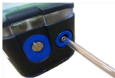
Figure 87: Connect Calibration Gas
