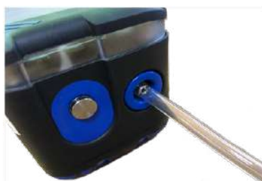
Figure 79: Connect Calibration Gas
