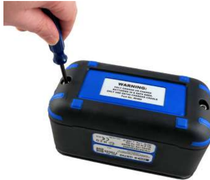
Figure 64: Battery Pack Removal
