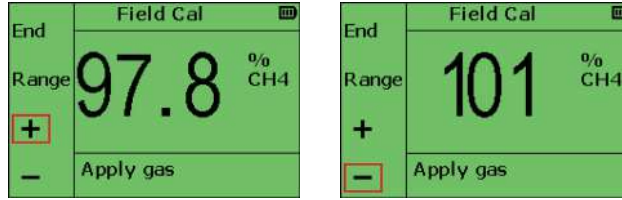
Figure 88: Field Calibration - Adjustment
