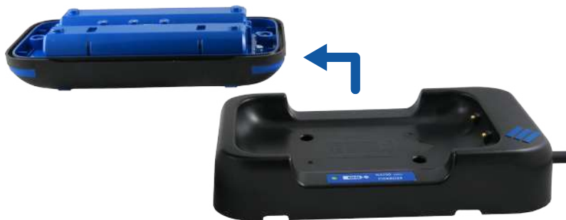
Figure 68: Battery Pack Charging
