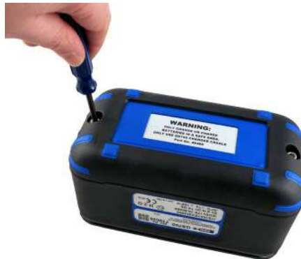
Figure 56: Battery Cover Removal
