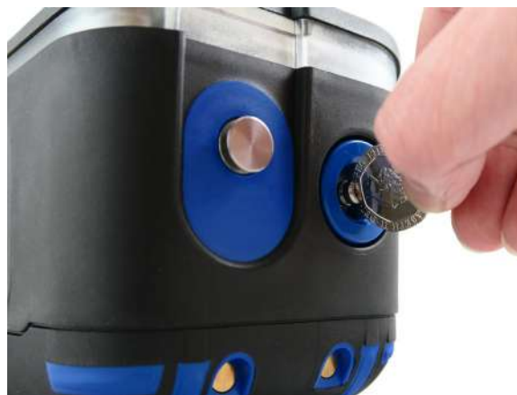
Figure 70: Inlet Nozzle Removal
