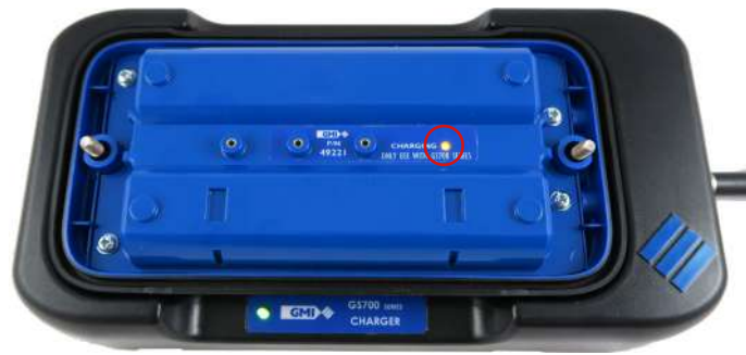
Figure 67: Battery pack LED
