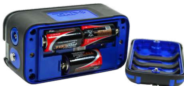
Figure 57: Battery Cover Removal
