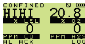
Figure 21: Confined Space Display (in alarm)
