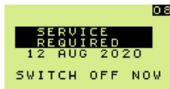
Figure 13: Service Due - Switch Off
