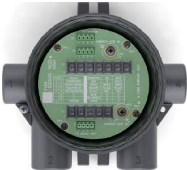
Figure 23 Junction Box Electrical Connections
