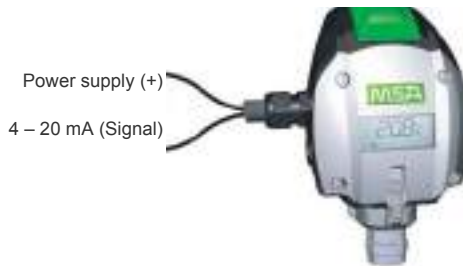
Fig. 7 2-wire connection - PrimaX I
