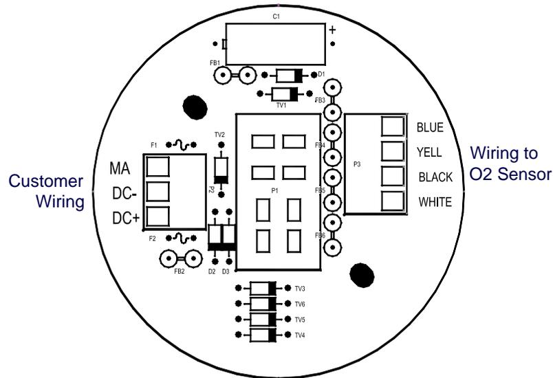
Figure 3 Base connector board
