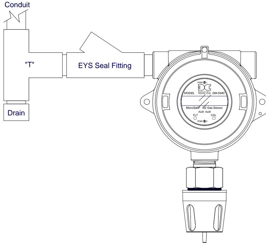
Figure 6 Typical Installation
