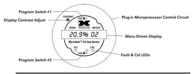
**NOTE**: If, after entering the calibration or program menus, there is no interaction with the menu items for more than 30 seconds, the sensor will return to its normal operating condition.
