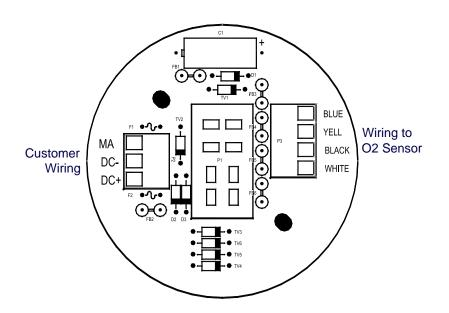
Figure 3 Base connector board
