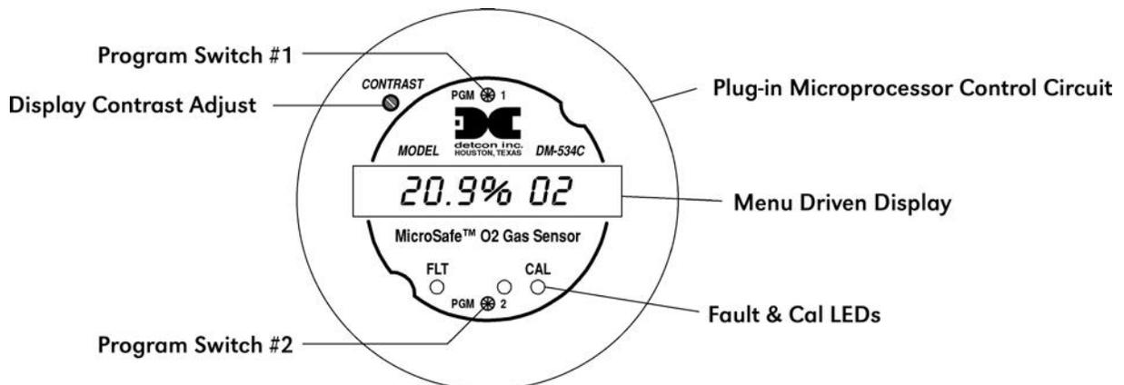
**Figure 2** Microprocessor Control Circuit
