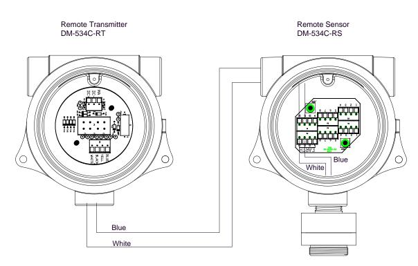
Figure 9 Remote mounting application
