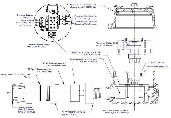
Figure 11 Spare parts diagram
