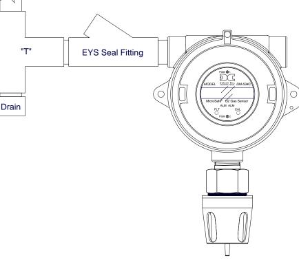
**Figure 6 Typical Installation**
