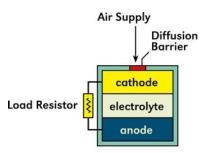
Figure 1 Construction of Galvanic Cell
