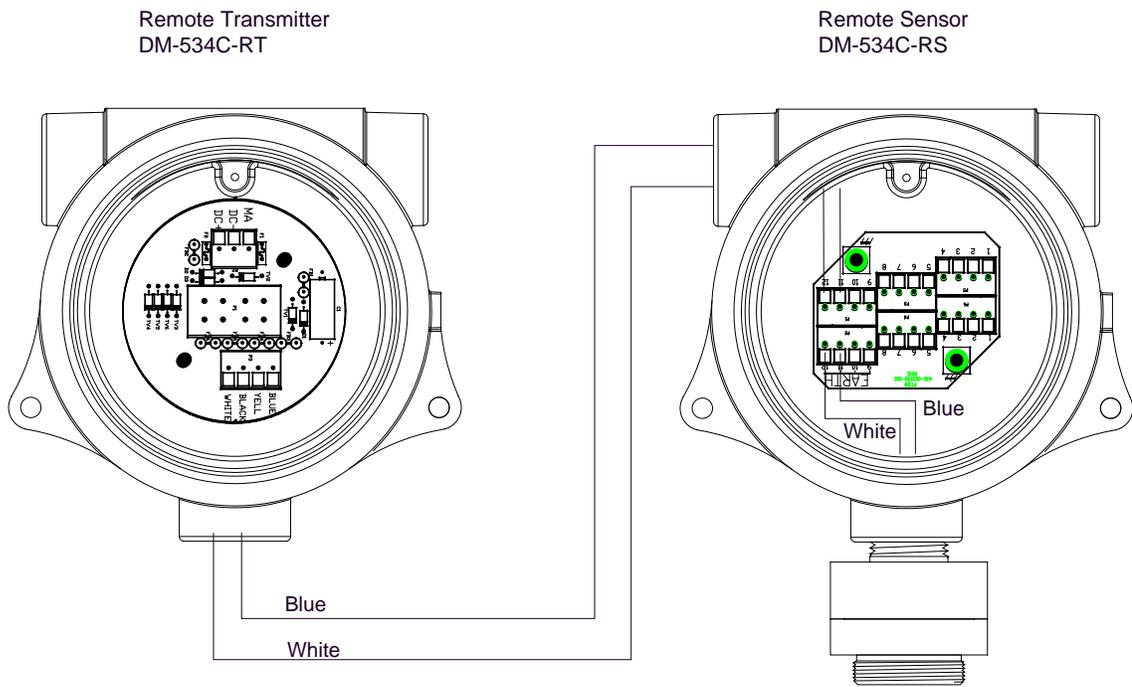
**Figure 9** Remote mounting application
