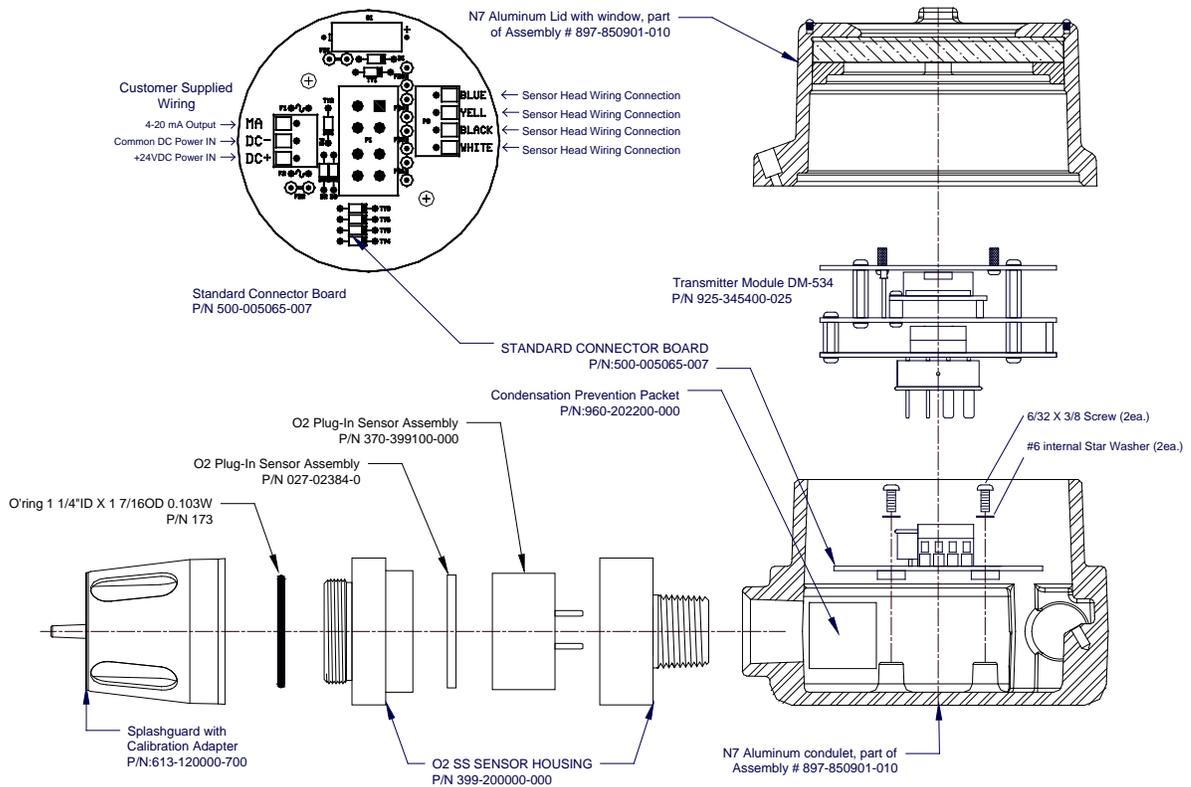
**Figure 11** Spare parts diagram
