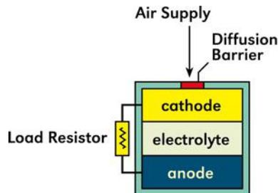
**Figure 1** Construction of Galvanic Cell
