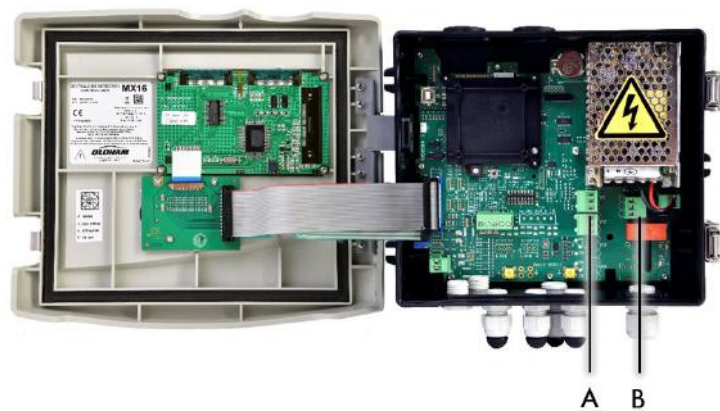
Figure 14: Internal alarm relays (A) and fault relay (B) terminals
