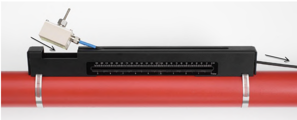
Figure 13 Installing downstream (blue) transducer
