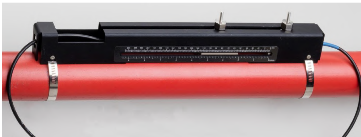
Figure 17 Lowering transducers onto pipe
