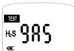
Figure 4-2: Manual Bump Test - Apply Gas
