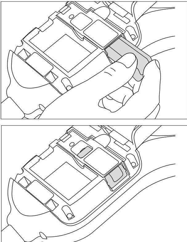
If you have difficulty inserting the cartridge please push it fully into place and hold for 3-5 seconds
