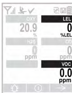
Toggle Display is for LEL and VOC sensor to alternate between LEL and VOC reading and their CFs. ProRAE Studio II allows other MultiRAE instruments to toggle the display for PID and LEL readings and CFs.
