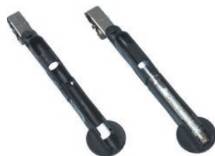
Direct indicating diffusion tube in holder
