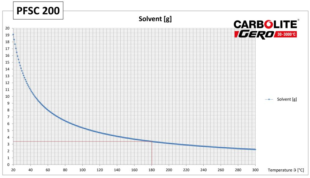
The steam volume of product PFSC200 is 248L. The maximum amount of solvent which can be placed in the oven at 180°C is approx. 3.39 g. At 20°C approx. 19.1 g solvent may be placed in the oven. The lower explosion limit used LEL =  $40 \text{ g/m}^3$ ; maximum concentration of flammable solvents  $c_{LEL} = 25\%$ ; theoretical vapourisation time  $t_0 = 2.58 / 9$ ; minimum exhaust flow  $Q_{min. 9} = 10 \text{ m}^3/h$ .
