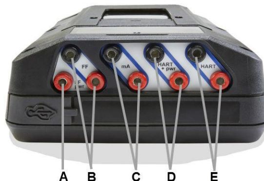
Figure 2-5: Device Communicator Plus communication module
