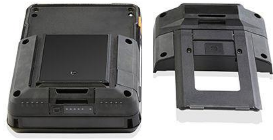
Figure 2-7: Trex unit with the communication module removed
