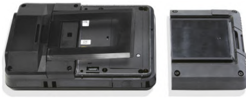
Figure 2-9: Trex unit with the power module removed
