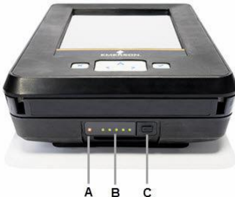
Figure 2-8: LEDs showing approximately 100 percent charge
