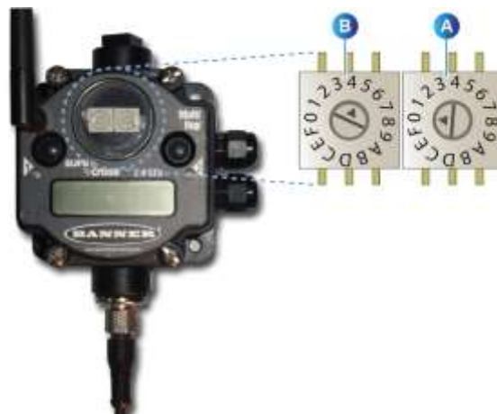
Figure 51: configuring the master receiver's address to @50.
