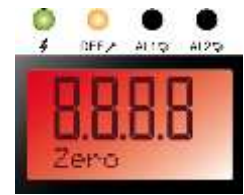
Figure 55: display in the event of a fault.
