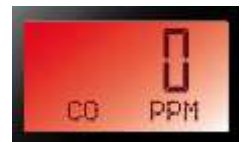
Figure 54: display under normal operating conditions.
