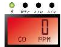
Figure 8: display sequence at start-up.
