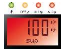
Figure 56: detection of high LEL concentration.
