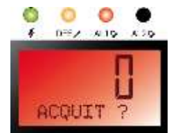
Figure 57: press ENTER on the reading to acknowledge an alarm.
