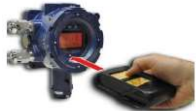
Figure 12: the remote control pointed toward the OLCT 80 .
