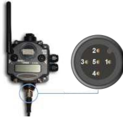
Figure 46: connecting the master receiver's 5-pin connector.
