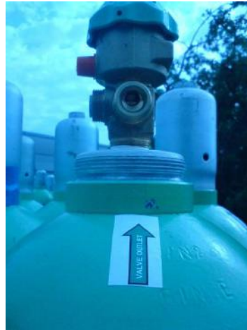
Typical marking of valve outlet port.
