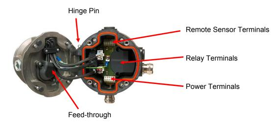
Dräger Polytron 5000 with e-Box attached
