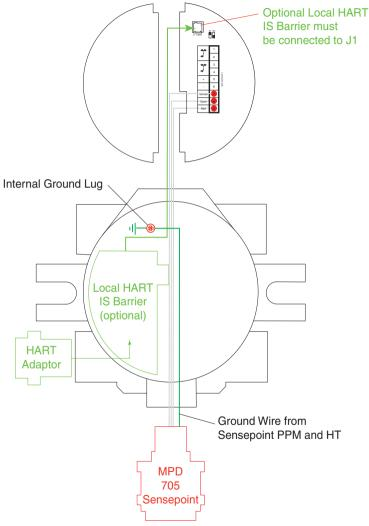
Figure 46. mV Personality Wiring
