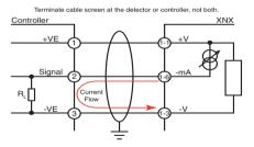
Figure 37. Source wiring for XNX
