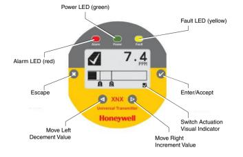
Figure 11. Front panel display of the XNX transmitter
