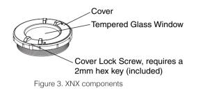
A tempered glass window requires the use of the supplied magnetic wand/screwdriver to activate the four user interface switches that are located on the front of the display module. This allows for nonintrusive setup and operation.
