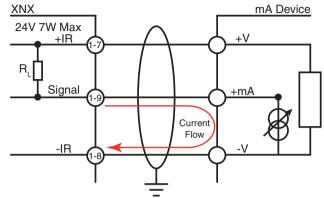
Figure 49. XNX mA input sink configuration
