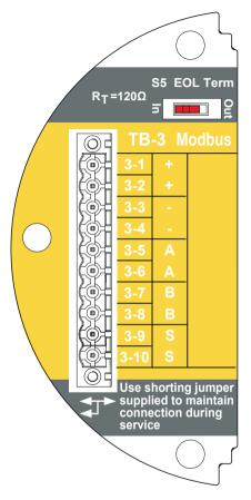
Figure 248. Modbus connections
