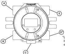
While relay wiring can use any available cable/conduit port in the XNX enclosure, do not use the same cable/conduit port for both relay reset and relay signal lines to avoid electrical noise.
