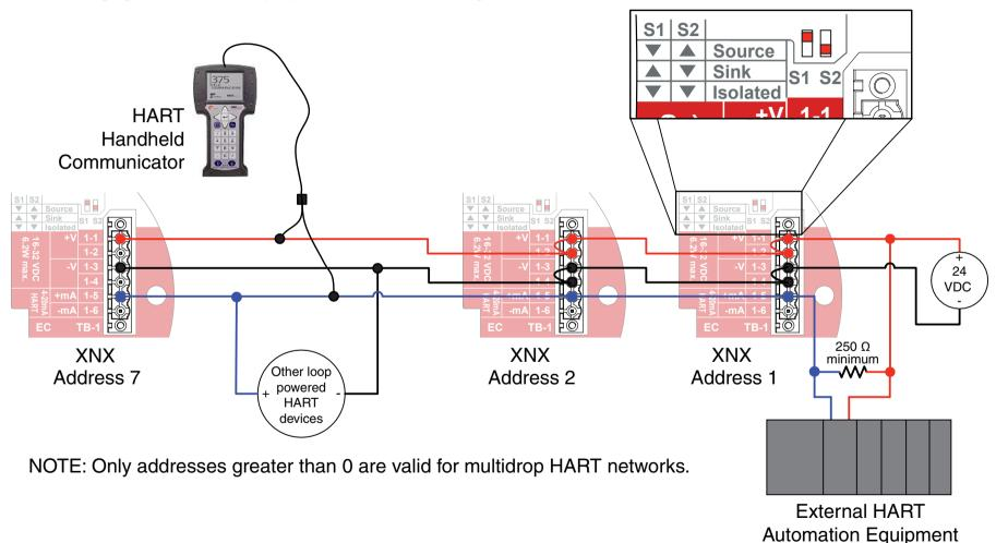
Figure 236. XNX Multidrop HART Network Wiring - XNX Sink
