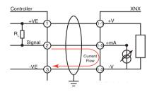
Figure 36. Sink wiring for XNX
