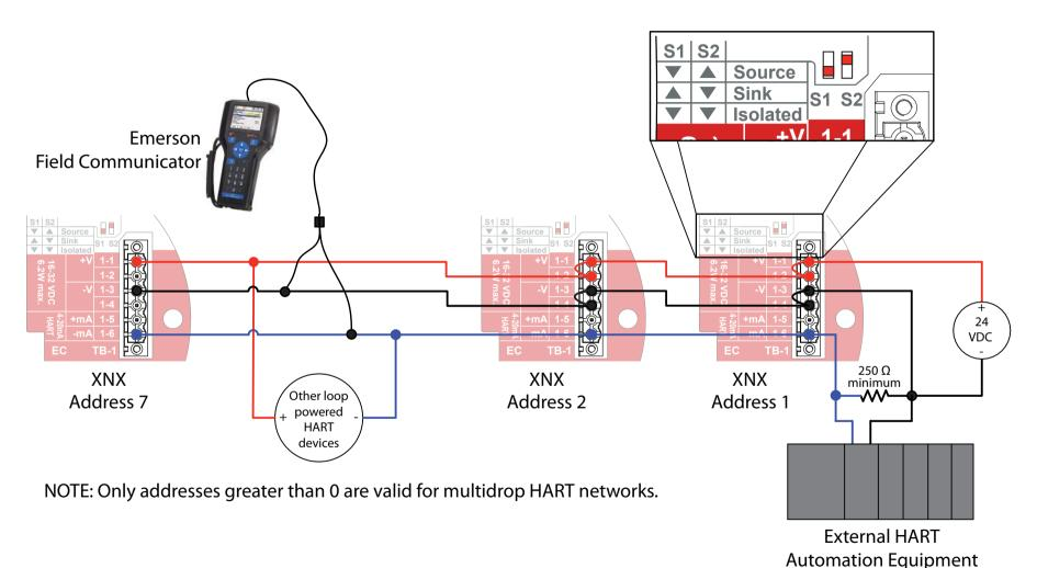
Figure 237. XNX Multidrop HART Network Wiring - XNX Source
