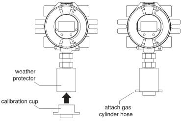
Figure 203. Attaching the Calibration Cup
