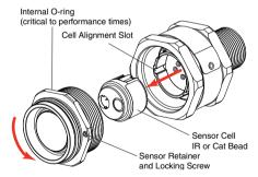
Figure 226. Removing the Plug-in Sensor
