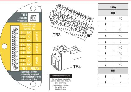
Figure 59. XNX Relay Option Board Terminal Blocks
