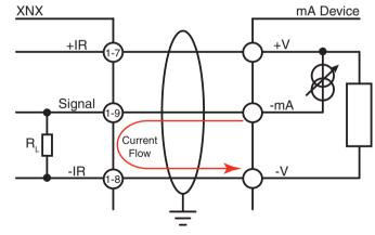
Figure 50. XNX mA input source configuration
