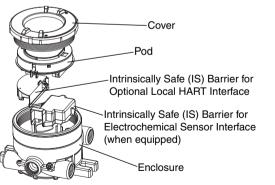
Figure 2. XNX Exploded View
