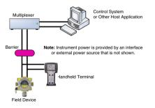
Figure 233. HART Point-to-point Mode
