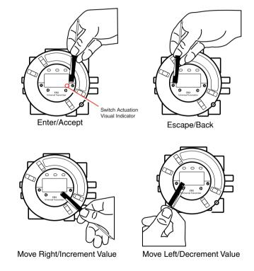
Figure 9. Using the magnetic wand
