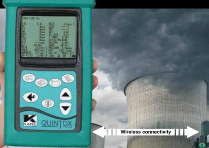
Independently tested by TÜV SUD to **EN50379** the new **KANE9206 Quintox** is a cost effective & versatile emissions monitoring solution.
